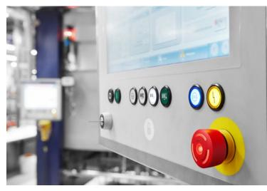
PHYSICAL SWITCH Figure 1: E-stop switches are just one of the components of the safety system. (Source: EAO)
