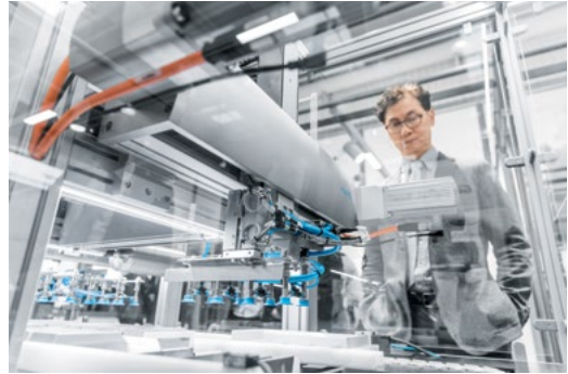
Figure 2: This pick-and-place gantry has flexible motion profile electric slides and pneumatically powered vacuum gripper.
