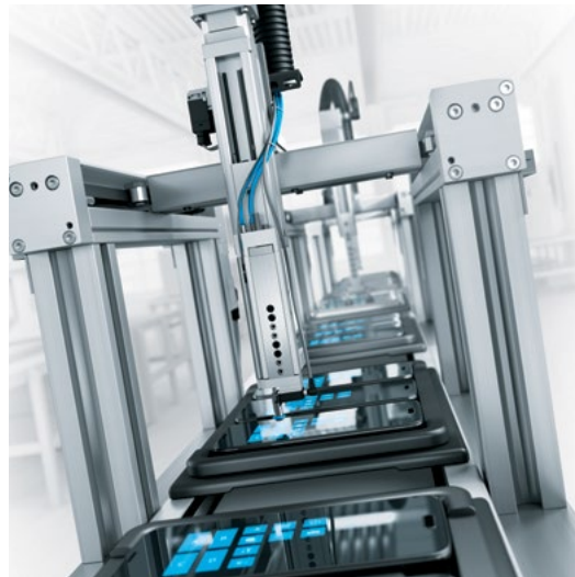
Figure 4: This electric light assembly features a combination of electrically powered slides featuring precise motion and pneumatically powered vacuum grippers for assured damage-free grip.
