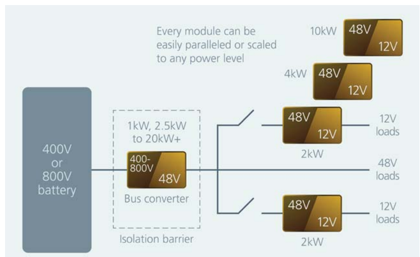
6. Fully electric vehicles can take advantage of the same hybrid-electric modular approach, with only the addition of an upstream fixed-ratio converter.
