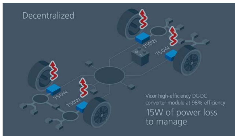
4. Decentralized 48-V architectures reduce losses by distributing lower currents and generating less heat; Vicor has developed converters that are 98% efficient.
