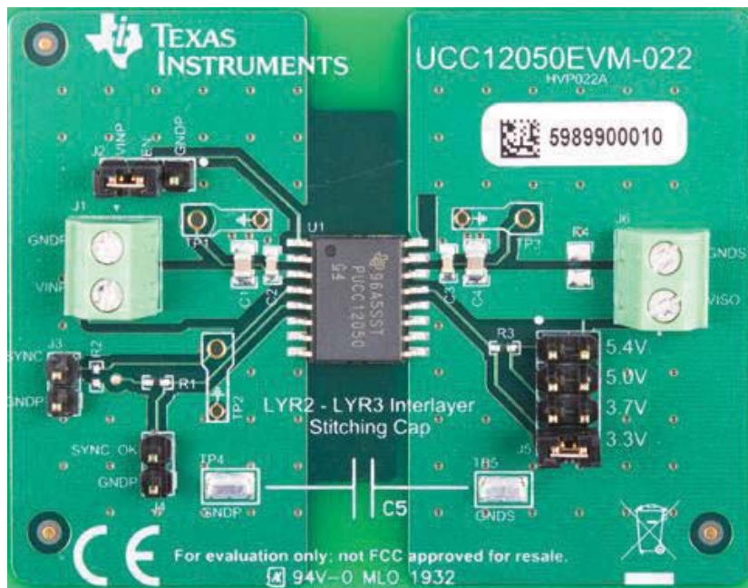
1. By integrating an isolation transformer into its package, TI's UCC12050 requires up to 80% less PCB space than a conventional solution. (Courtesy of Texas Instruments)
