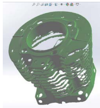
13. After running through the ScanTo3D wizard, SolidWorks can come up with a haggard but usable mesh representation of the motorcycle cylinder.
