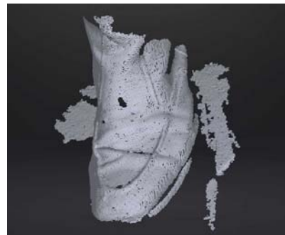
2. I could not get any points scanned of a black Harley cylinder. Then I accidentally moved the scanner past my shoe that was speckled with white paint.
