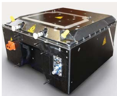
2. Formula E cars use the same battery pack. Battery-management and regenerative-braking support can be key to a team's success.
