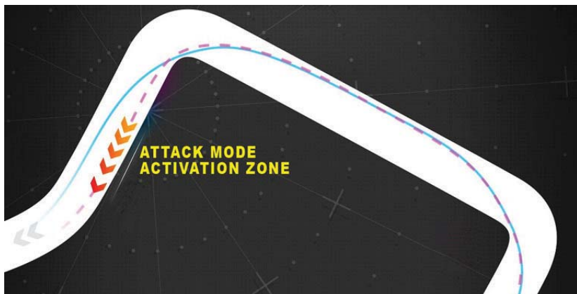
3. Formula E attack mode requires the car to move through a designated area that normally forces the driver to slow down or cover more ground to offset the later advantage.
