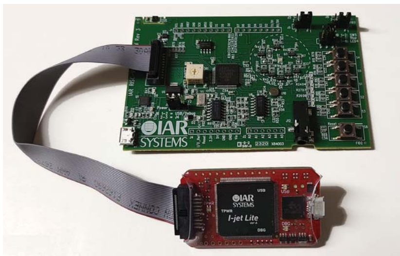
IAR's development board is built around the GD32VF103RBT6 RISC-V microcontroller from GigaDevice Semiconductor. The I-Jet Lite provides JTAG support.
