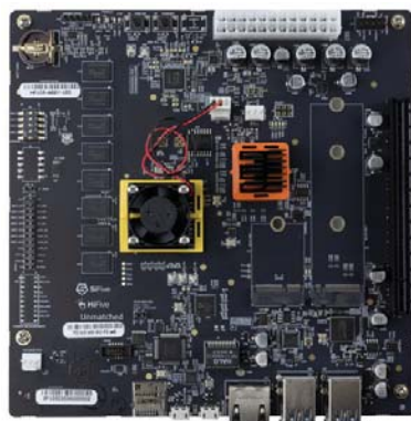
SiFive's HiFive Unmatched Mini-ITX motherboard features an FU740 SoC with four SiFive U74 cores and one SiFive S7 core.
