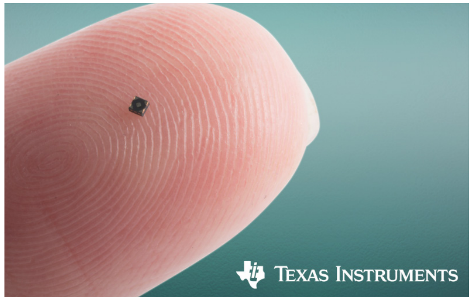
1. Better not sneeze: Aimed at IoT and personal electronics applications, the TLV9061 consumes only 0.64\text{mm}^2 and is the world's smallest op amp. (Source: Texas Instruments)
