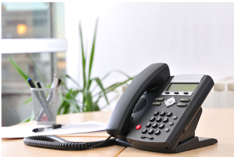
2. A voice-over-IP (VoIP) telephone was a typical node supported by power-over-Ethernet (PoE), requiring only a single cable connection to a PoE switch. (Dreamstime)
