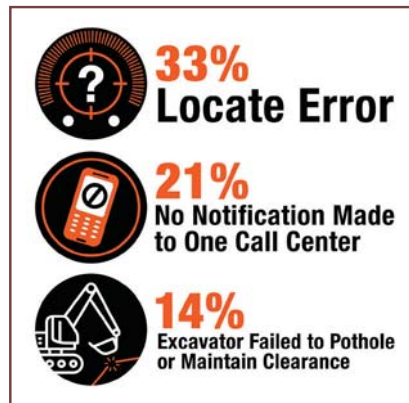
FIGURE 1. Leading root causes of damages to underground telecommunication lines, according to the 2021 DIRT report.
