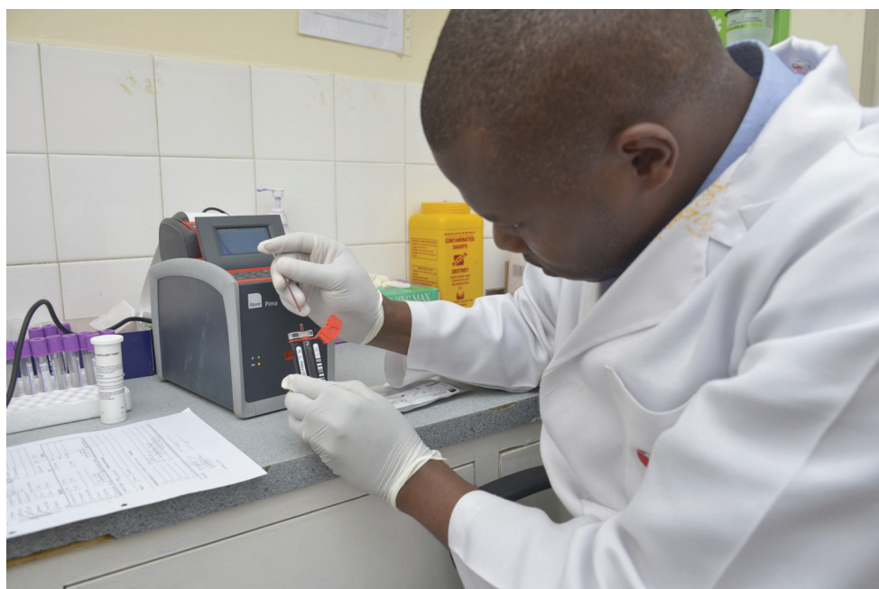
A Pima CD4 user ensures that the cartridge's sample capillary is completely filled, that no air bubbles are introduced, and the specimen is visible in the control window of the cartridge. (Photo courtesy of CHAI)
