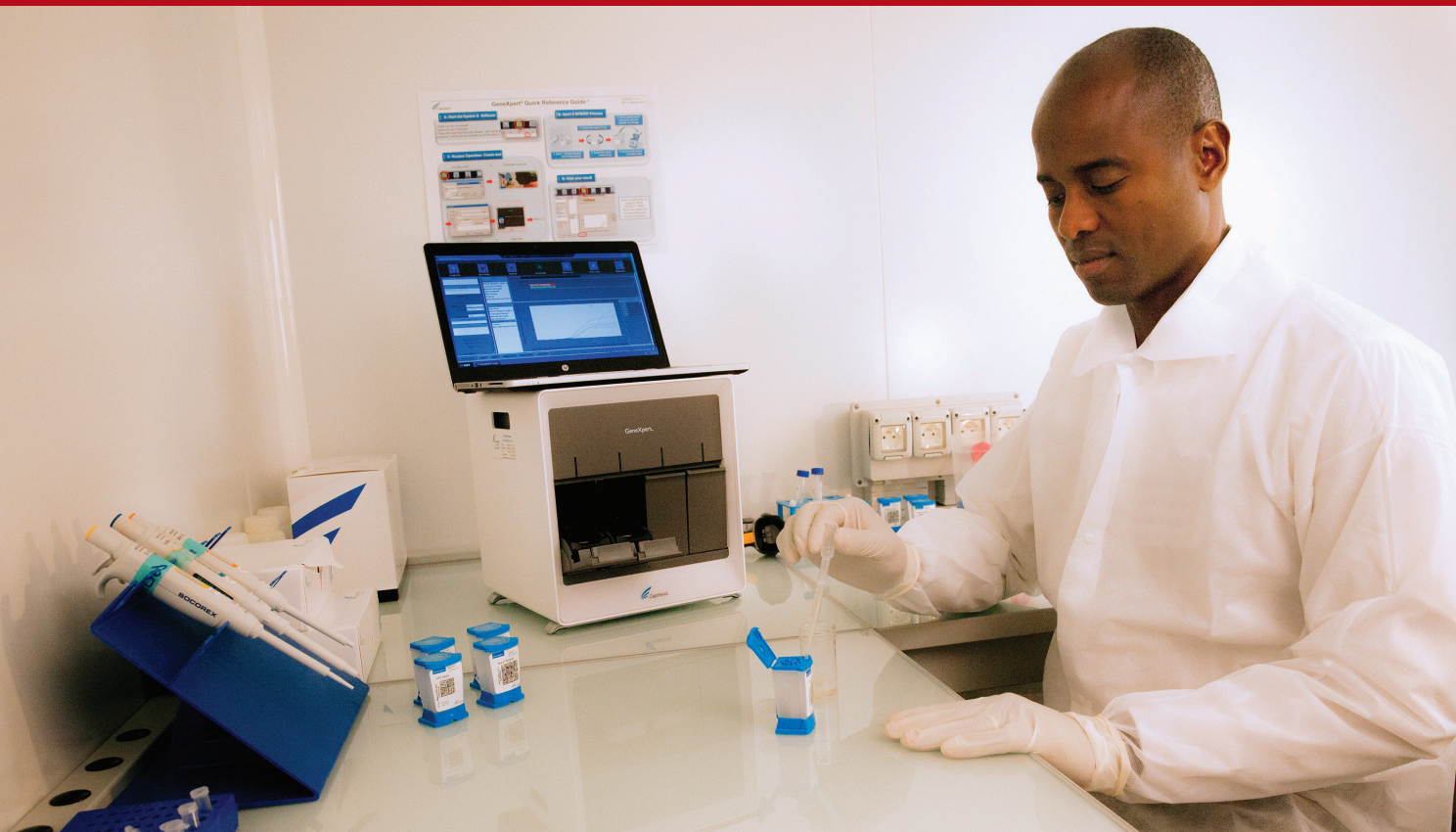
POC instruments are available in multiple configurations based on the number of cartridges that can be analysed simultaneously. Capacity can vary from 1 test per run to 80 tests per run, depending on the instrument. (Photo courtesy of Cepheid)
