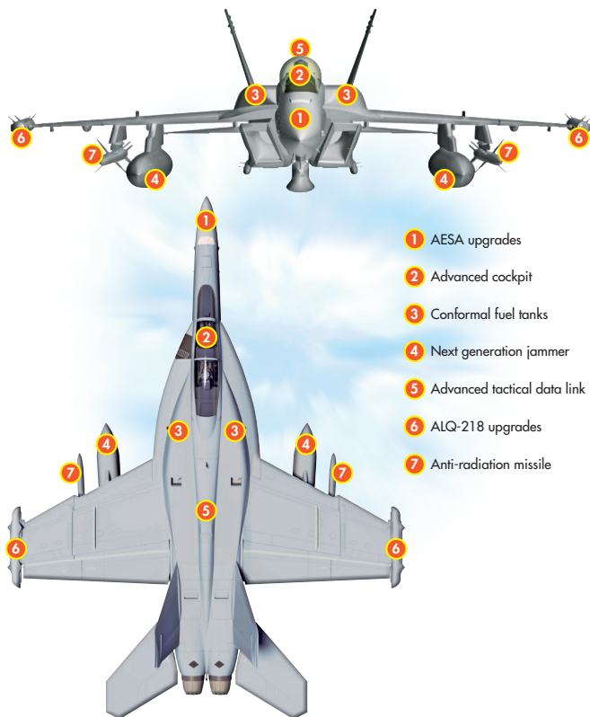
2. Many design configurations are possible with the modular mounting systems on the EA-18G platform. Additional space also is available, thanks to the move toward conformal fuel tanks on the dorsal side of the platform. (Courtesy of Raytheon)
