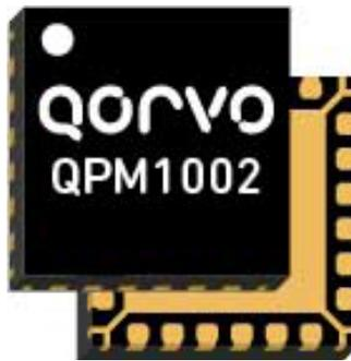
2. Qorvo's QPM1002 T/R FEM serves radar applications from 8.5 to 10.5 GHz. (Courtesy of Qorvo)
