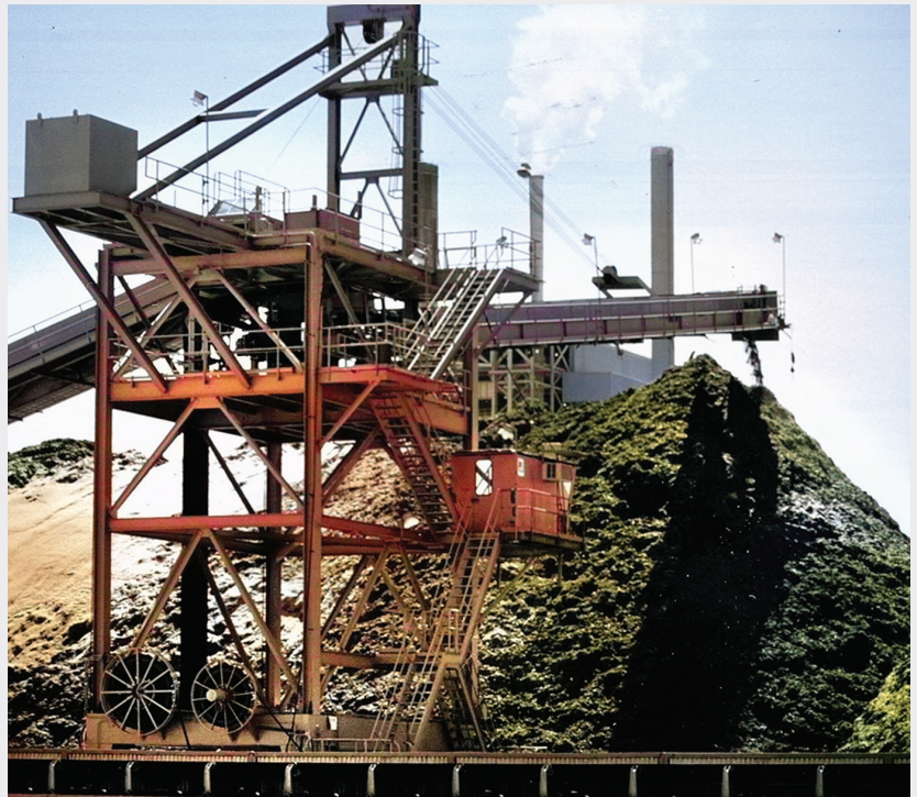
Figure 1. Conveyor blockage, damaged bearings or other failed components in the driven equipment can mechanically overload a motor, causing it to trip during startup.
