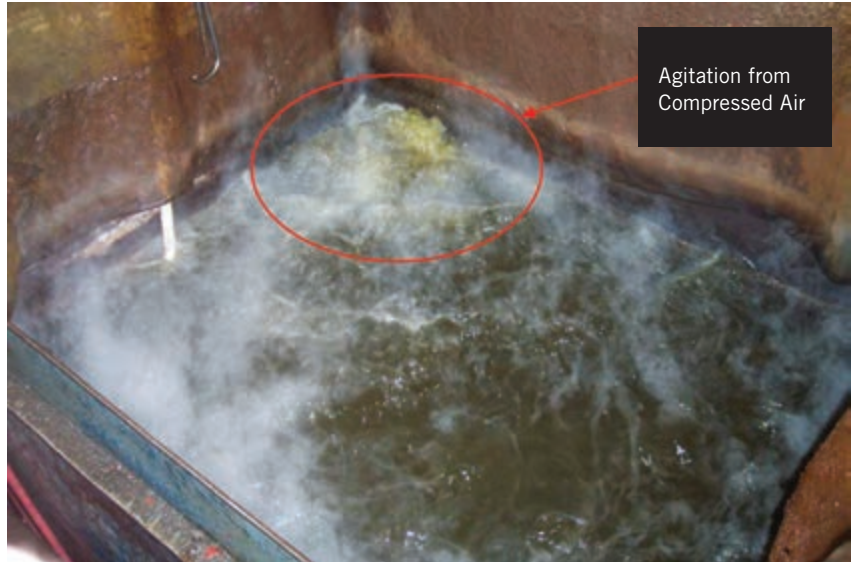
Figure 1. Agitation was measured at 10 cfm of 100 psi compressed air.
