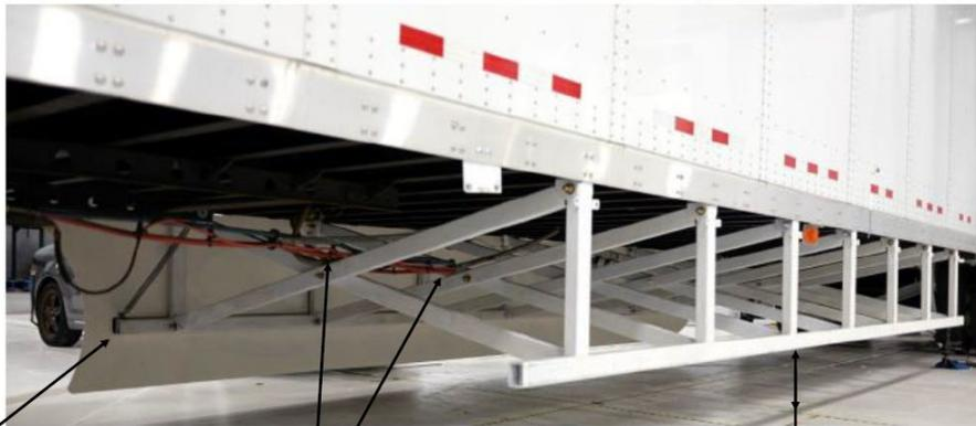
The rigid bracing behind aerodynamic trailer side skirts have instituted DOT safety recalls of specific side-skirt designs.
