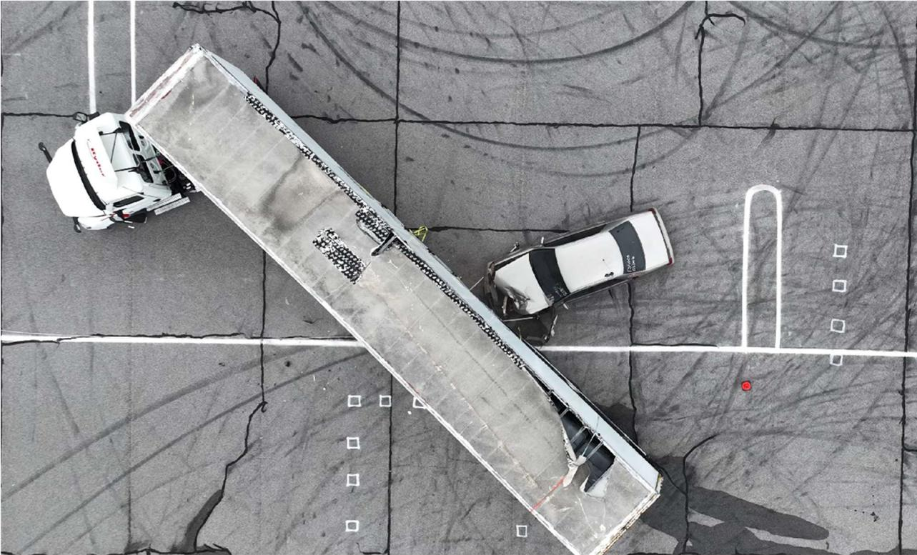
90 Degree Angle **Behind Axles** Test, Chevrolet Malibu, 35 mph, SafetySkirt Side Guard, 8/2023
