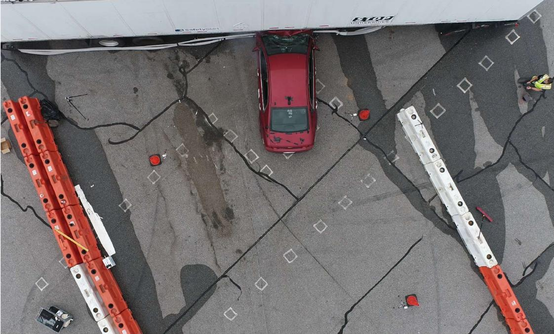
45 Degree Angle Test, Ford Fiesta, 40 mph, Angelwing Side Guard, 8/2023
