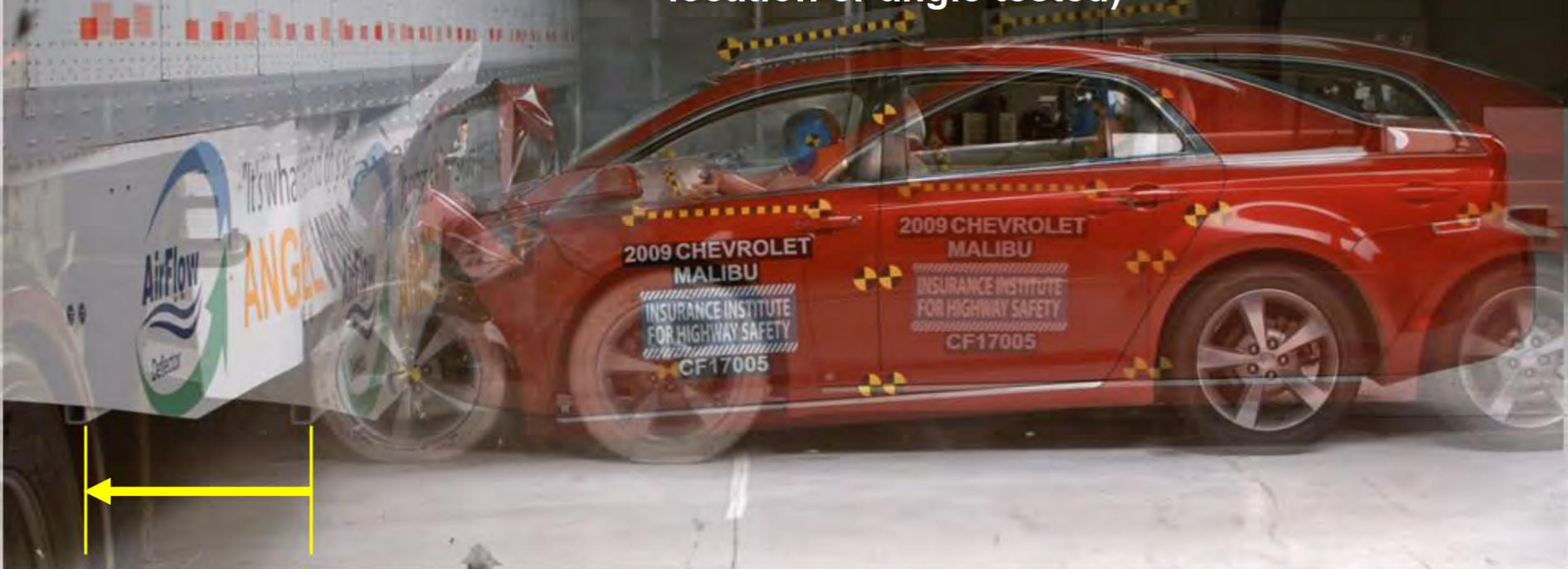
**Excessive slide (approximately 24") from impact of trailer (poor test boundary condition – lightly loaded trailer, smooth floor).**
