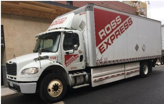
Figure 8: Photo of a Single-Unit Truck (SUT) with Aero Side Guard
