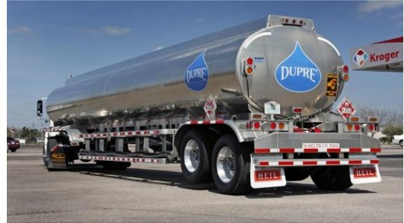
Figure 7: Photo of a Combination Truck (CT) with Rail Side Guard
