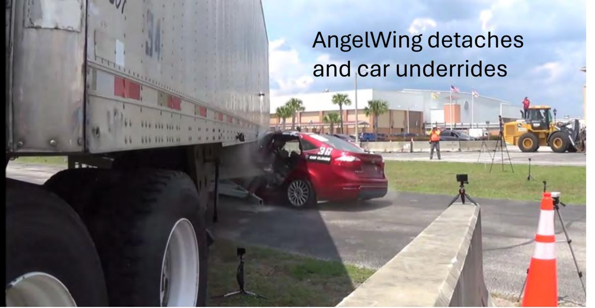
Combined (45 degree) longitudinal and lateral impact caused AngelWing to detach
