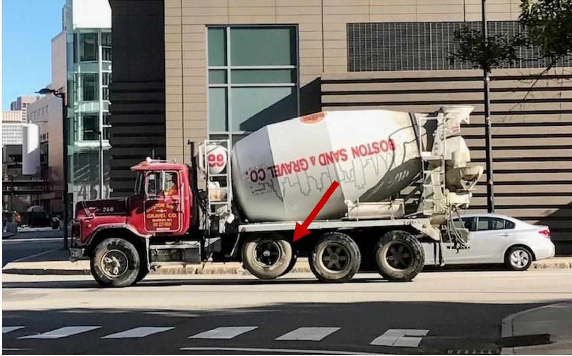
**Figure 48: Truck with a lift axle. (Source: Volpe)**
