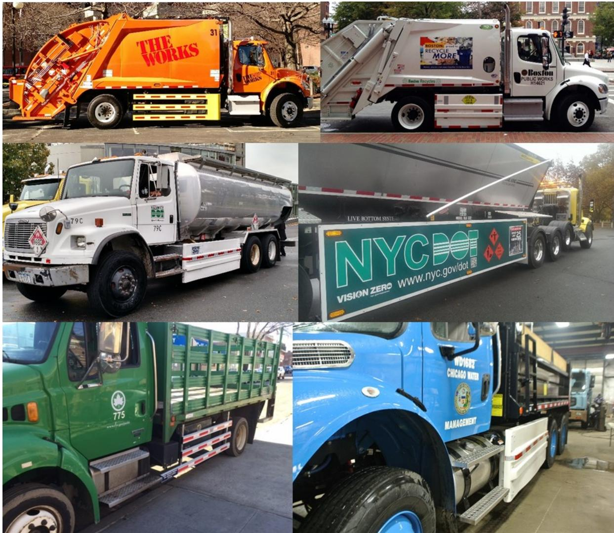
Figure 5: Images of side guard-equipped trucks in Cambridge (top left), Boston (top right), New York City (middle left, middle right, and bottom left), and Chicago (bottom right) (Source for Chicago: Rosanne Ferrugia; Boston: Kristopher Carter; others: Volpe)
