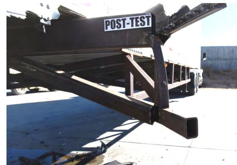
**UTM Side Impact Guard was not effective when impacted at one end. This is the only test we know of conducted at 30% (car to guard) overlap.**
