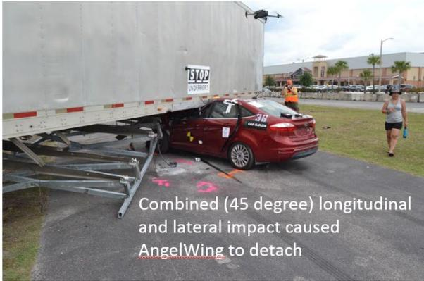
Combined (45 degree) longitudinal and lateral impact caused AngelWing to detach
